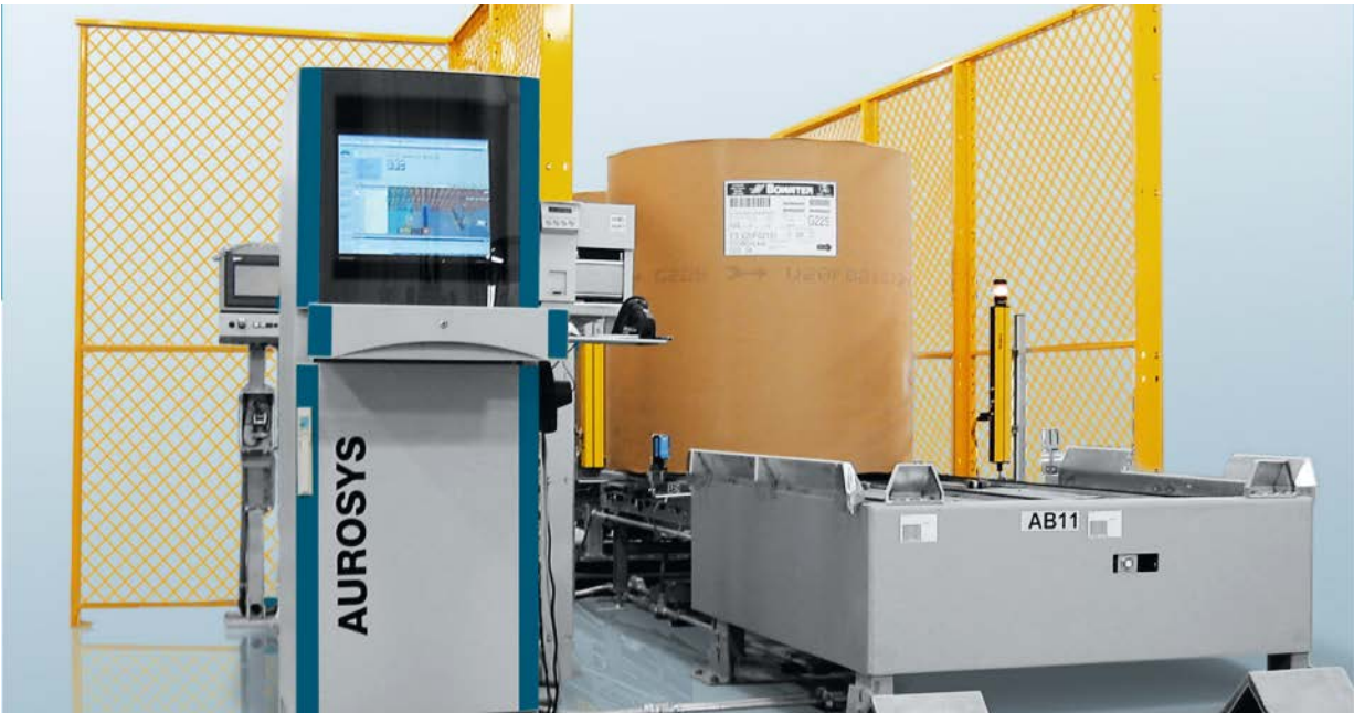
➤ As an automated, customized logistics solution, AUROSYS takes care of automatic truck unloading, storage, unpacking and preparation of the paper rolls for gluing, right through to automatic supply to the reelstands and the disposal of residual rolls, cores and waste paper.
