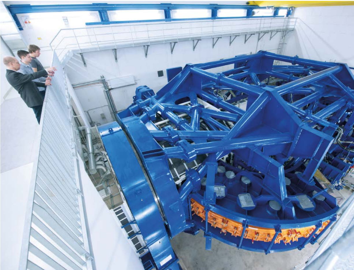
➤ HIT uses a gantry — a movable beam guidance system — that can rotate the beam exit 360° around the patient for optimal irradiation.
