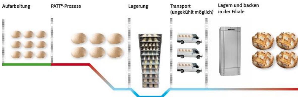
Fig. 6: Cooling chain of a bakery using the PATT process for the gentle freezing of dough pieces (Photo: KOLB KÄLTE)
