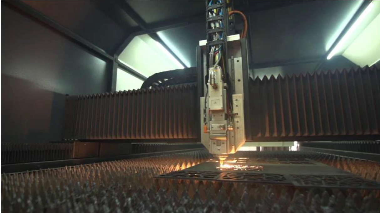
Fig. 5: View of the inside of the completely enclosed machine: highly dynamic XYZ positioning system with a laser cutting head (Photo: Accumech)
