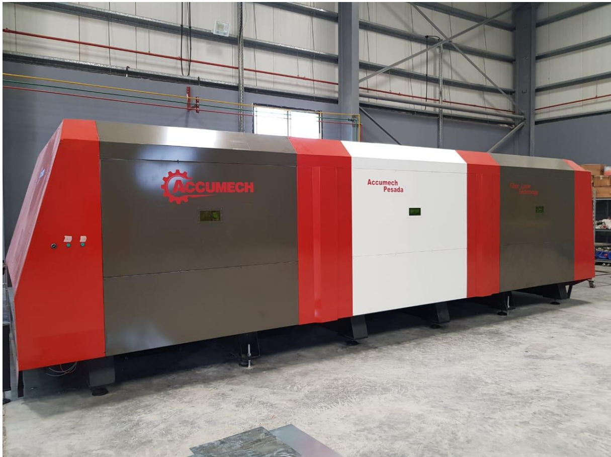
Fig. 1: PESADA CNC laser cutting machine and shuttle table (image: Accumech)
